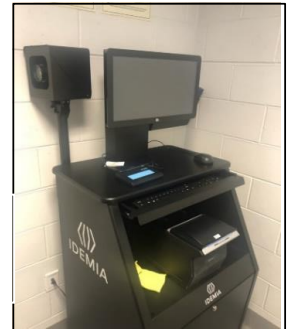
AFIS machine located in the booking area of the station.
