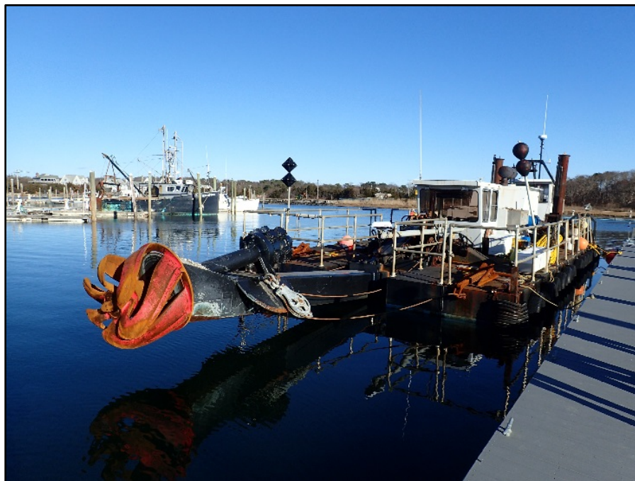
Figure 14. Hydraulic suction dredge cutter head (left) on the County dredge “Cod Fish”, January 2018.
