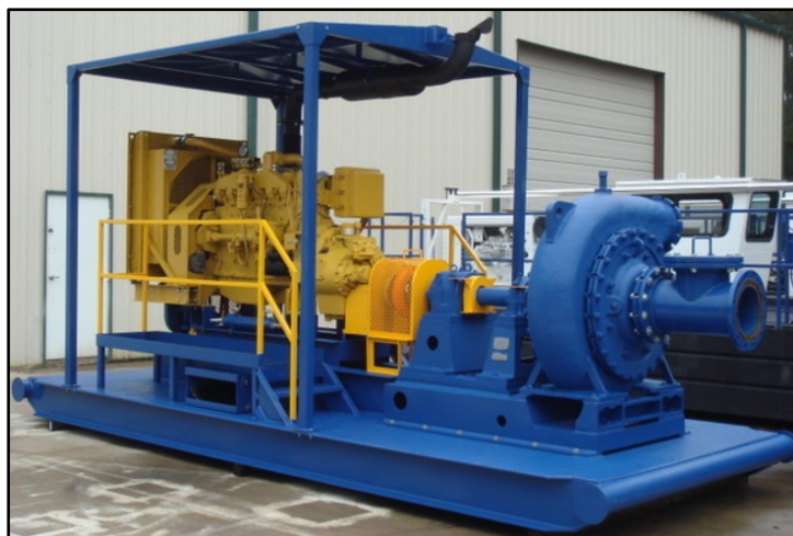
Figure 20. Typical skid-mounted hydraulic dredge booster pump. 29 June 2018, https://www.westerndredge.com/product/10in-cat-booster-pump/
