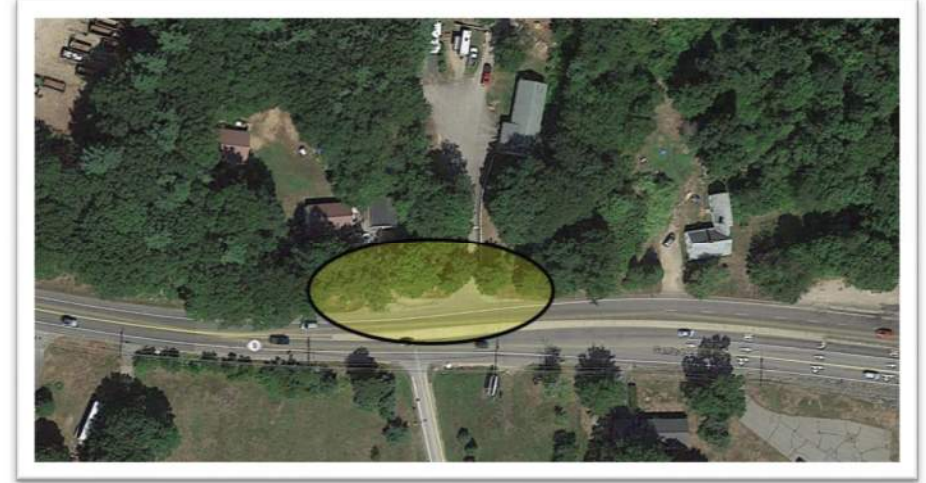
FIGURE 34: ACCESS MANAGEMENT DEFICIENCIES ALONG ROUTE 109 & 9 (SANFORD ROAD) BETWEEN INTERSECTION WITH SPENCER DRIVE AND CHAPEL ROAD
