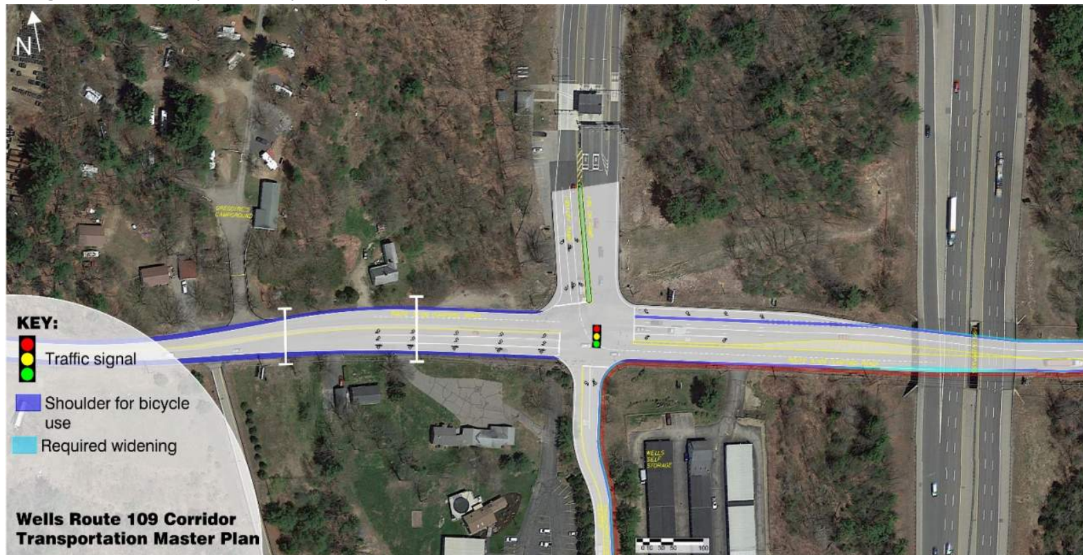
Figure 39: Recommended Improvements for the Intersection of Routes 109 and 9 (Sanford Road) and Turnpike Exit 19/Wells Transportation Center
