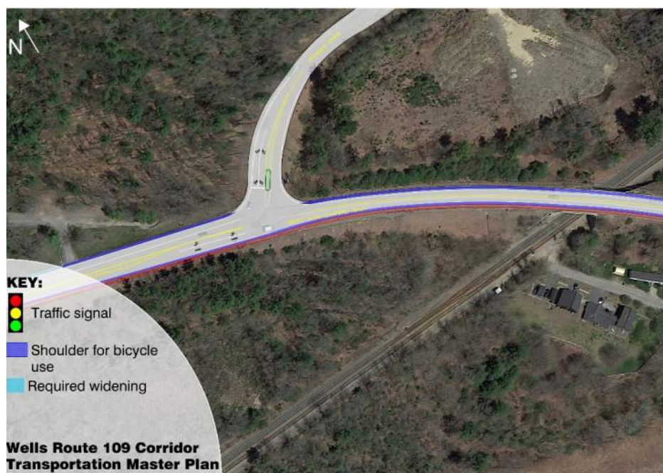
FIGURE 40: RECOMMENDED IMPROVEMENTS FOR THE INTERSECTION OF ROUTE 109 AND 9 AND SPENCER DRIVE
