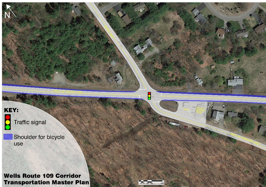
Figure 37: Proposed Improvement to the Intersection of Route 109 (Sanford Road) and Branch Road/Crediford Road
